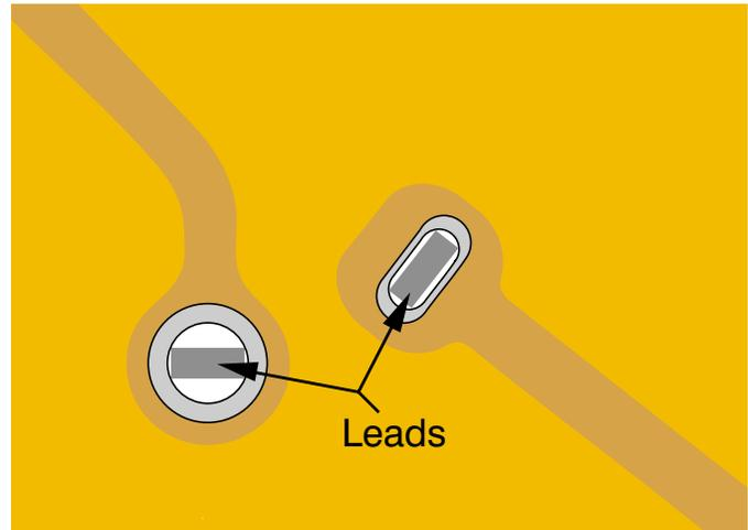
Round through-holes vs. slotted through-holes
