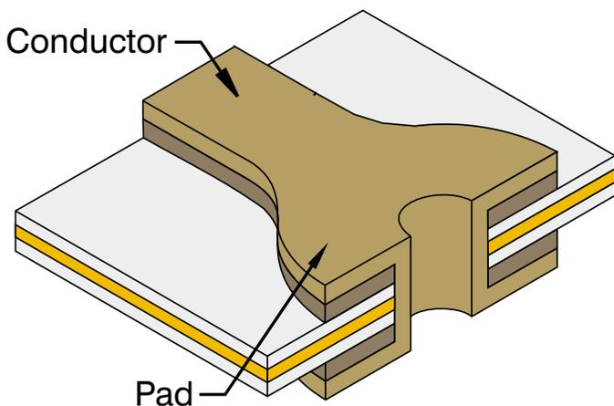
3. Copper is etched to create conductors and pads
