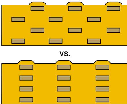
*Staggered conductors vs. I-beam effect*
