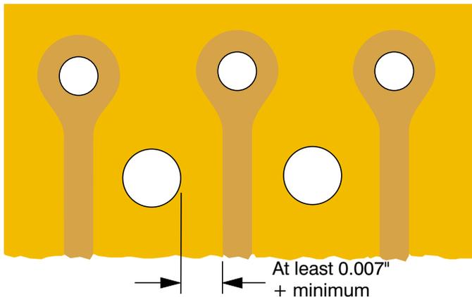
*Non-wiring hole at least 0.007" + minimum from conductor.*
