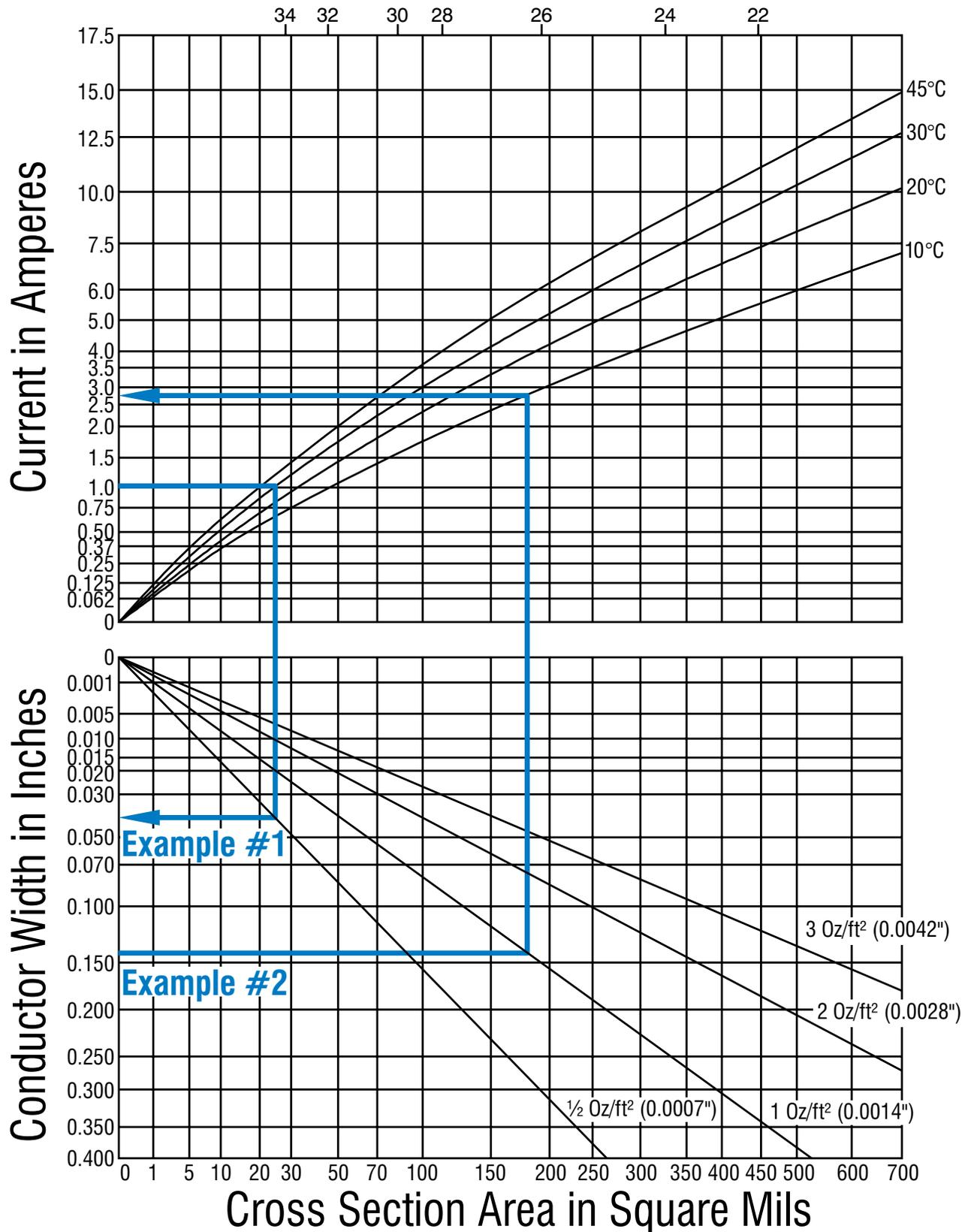
**Example #1:** A current of 1 amp with 1/2 oz. copper and 30°C temperature rise will require a conductor width of 0.040".
