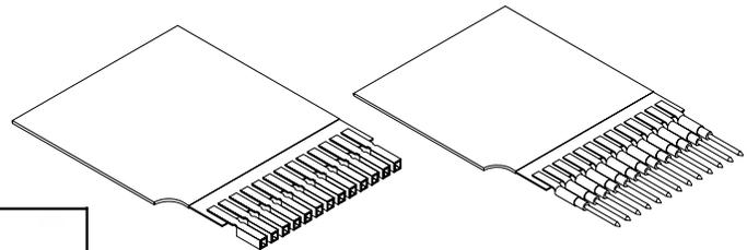
Crimped pins and sockets
