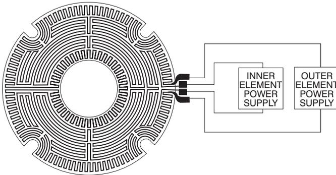
Custom dual-element heater for profile testing
