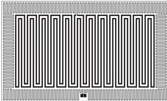
Heater profiled for higher wattage at edges
