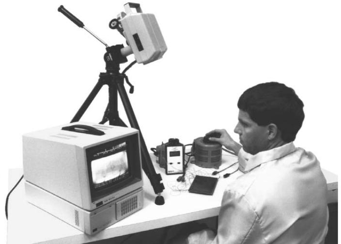
*Typical heater test and prototyping setup: Heater (with multiple elements), variable power sources, digital temperature indicator, and infrared thermal imager.*
