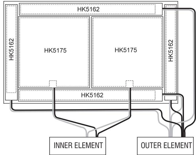
*Test setup for heater profiling analysis.*
