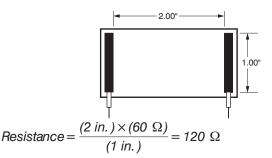
For instance, assume you have an ITO coating with a resistivity of 60  $\Omega$ /square. A 1" X 1" heater would have 60  $\Omega$ . And a 2" X 2" heater would have 60  $\Omega$ . Consider each 1" square as a resistor of resistance=R and use Kirchhoff's Current Law for series/parallel resistance circuits:
