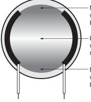
More current flow (power) where distance between bus bars is shortest.
