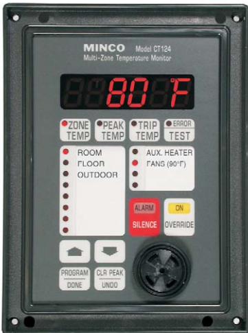
Override: Override has been pressed and is active. It has switched on the cooling fans wired to Relay 2 regardless of temperature.
