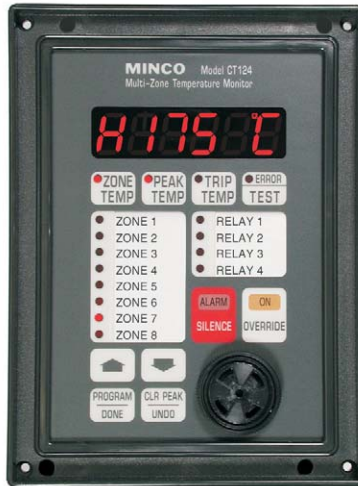
Peak temperature: Zone 7 has reached a high of 175°C since the last time peaks were cleared. The Clr Peak button will reset the peak to the current reading in Zone 7.
