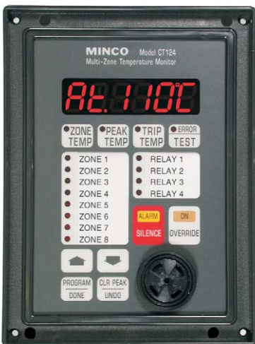
Program mode: The CT124 is in the program mode. The Alarm trip point (At) is set to 110°C. Press Up and Down arrows to change this number. Done to proceed to the next choice, or Undo to back up.
