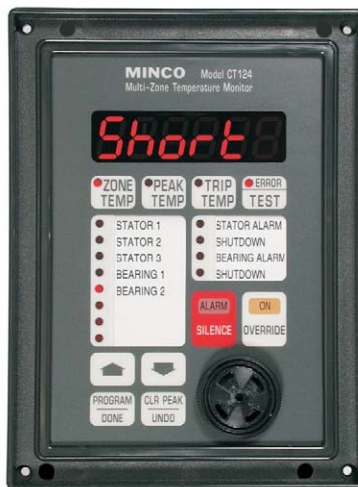
Input fault: Zone 5 has a short circuit. It is locked out; other zones operate normally.
