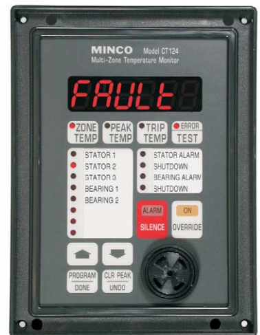
Intermittent fault: Zone 2 has experienced an intermittent short or open.
