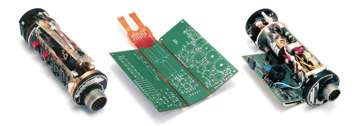
**Before:** A tangle of wires connects four circuit boards in this aircraft gauge.
