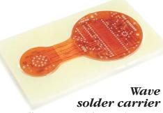
Stiffener material frames the circuit to hold it flat during wave solder. After soldering, just clip out and fold.
