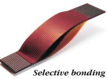
For better flexibility along circuit arms, individual layers are unbonded and allowed to flex freely. Each layer has its own substrate and cover.
