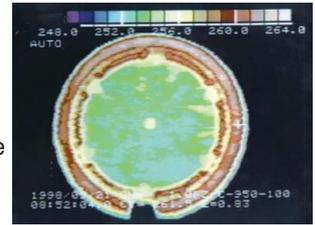
Thermal imaging does require line-of-sight access to heaters, which may not be possible under actual use conditions. Nevertheless, it is a valuable addition to the thermal designer's toolkit.
